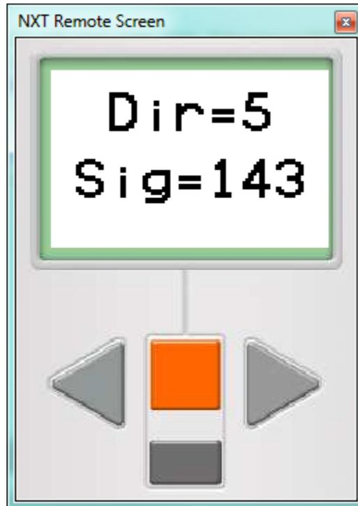
Figure 16 - RoboSeek.c Will Follow an AC IR Signal and Display the Direction and Max Intensity on the LCD
