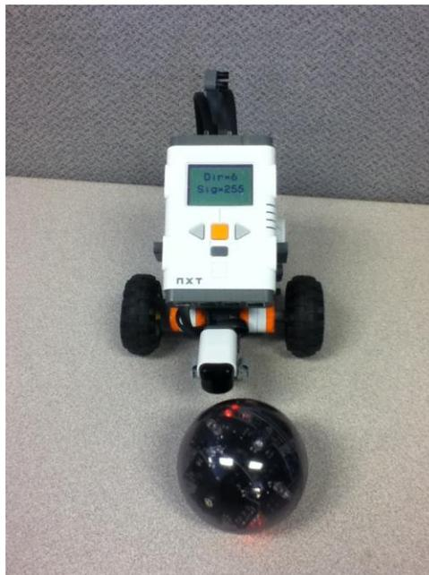
Figure 17 - Robot with IR Seeker and IR Soccer Ball
