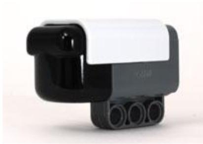
Figure 2 - HiTechnic IR Seeker v2
